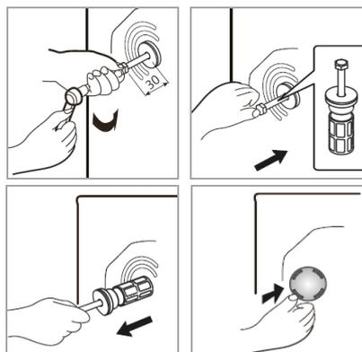
Remove the transport locking screws with a wrench. Insert the supplied transport locking covers.
